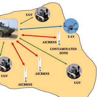
Sentry concept (manual) and would be networked to the SADSS of CBRN Centres at Battalion HQ, Brigade and above. The AICBRNS integrates into a single unit: • CBR Sensors/Detectors. Compact, lightweight and modular sensors, to detect and record agent parameters, (Agent identification, intensity, persistency, volatility, and hotspot locations). An operating range of 100m in battlefield conditions would be optimal. The detection would be point/ proximity detection on occurrence/release.
